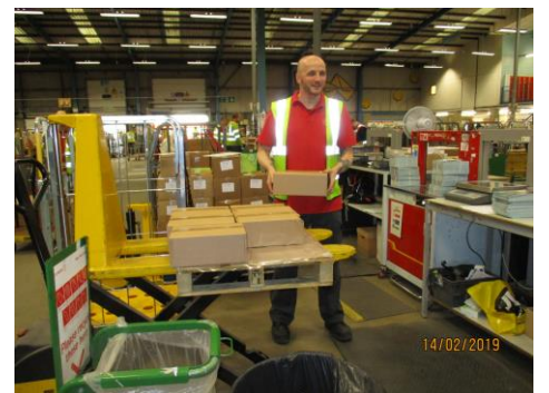
Dense boxes or bundles use a pallet lifter
